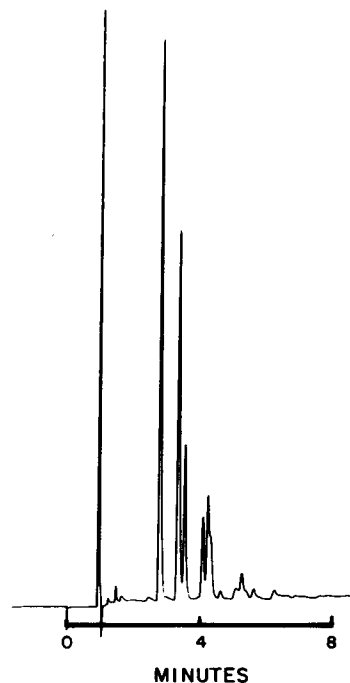
FIG. 6. Separation of triglycerides in sunflower seed oil. Column and conditions as in Figure 1.
